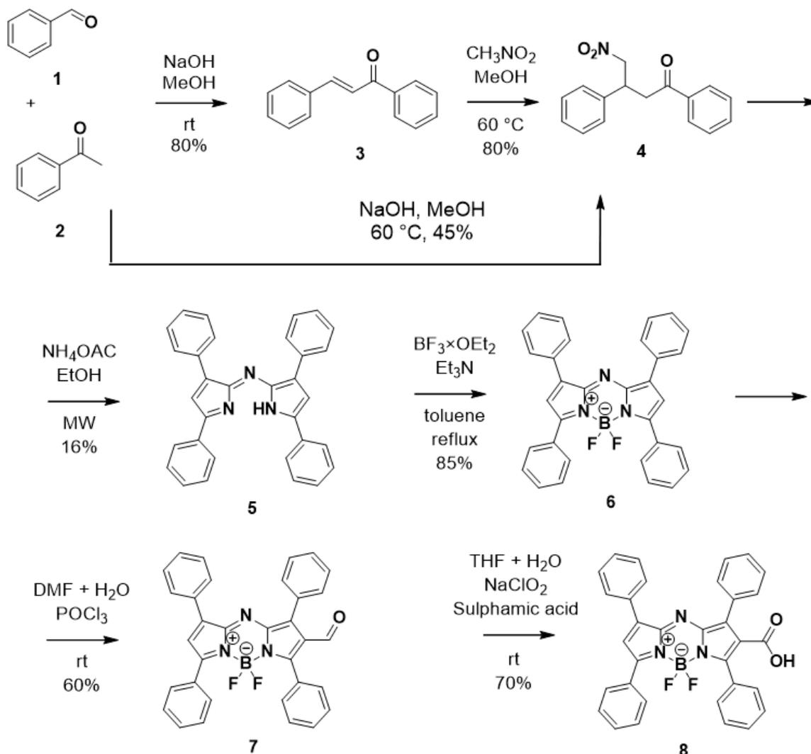
Scheme 1. Synthesis of the carboxylic acid derivative (**8**)
