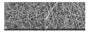
Figure 1. SEM images of PSFQ fibers obtained from solutions of 40% concentration in DMF (a) and NMP (b).
