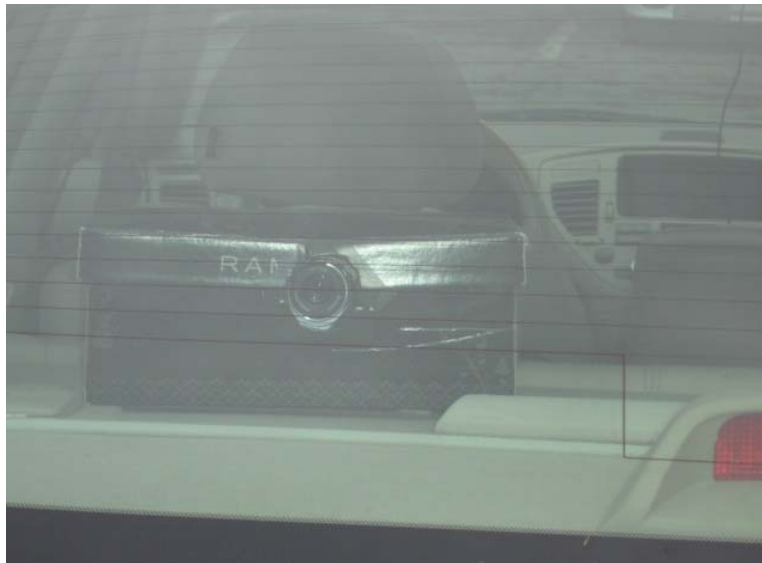
Figure 9: Disguised Digital Camcorder behind the Rear Windshield
