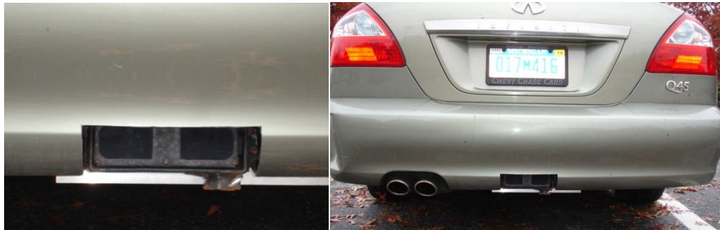
Figure 7: IR Sensor at the Center of Back Bumper
