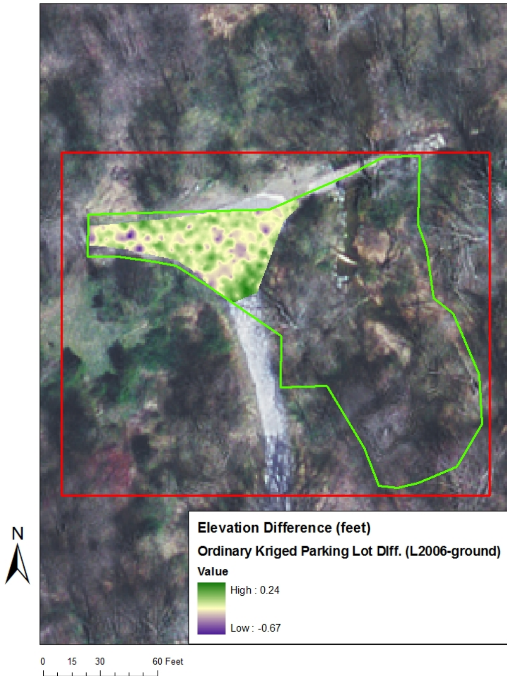
Figure 4-19. Ordinary Kriged parking lot difference raster (Kriged LiDAR 2006 raster minus kriged Ground-Surveyed raster over the parking lot surface). Mean elevation difference for (Lidar-Ground) is -0.15892 ft.
