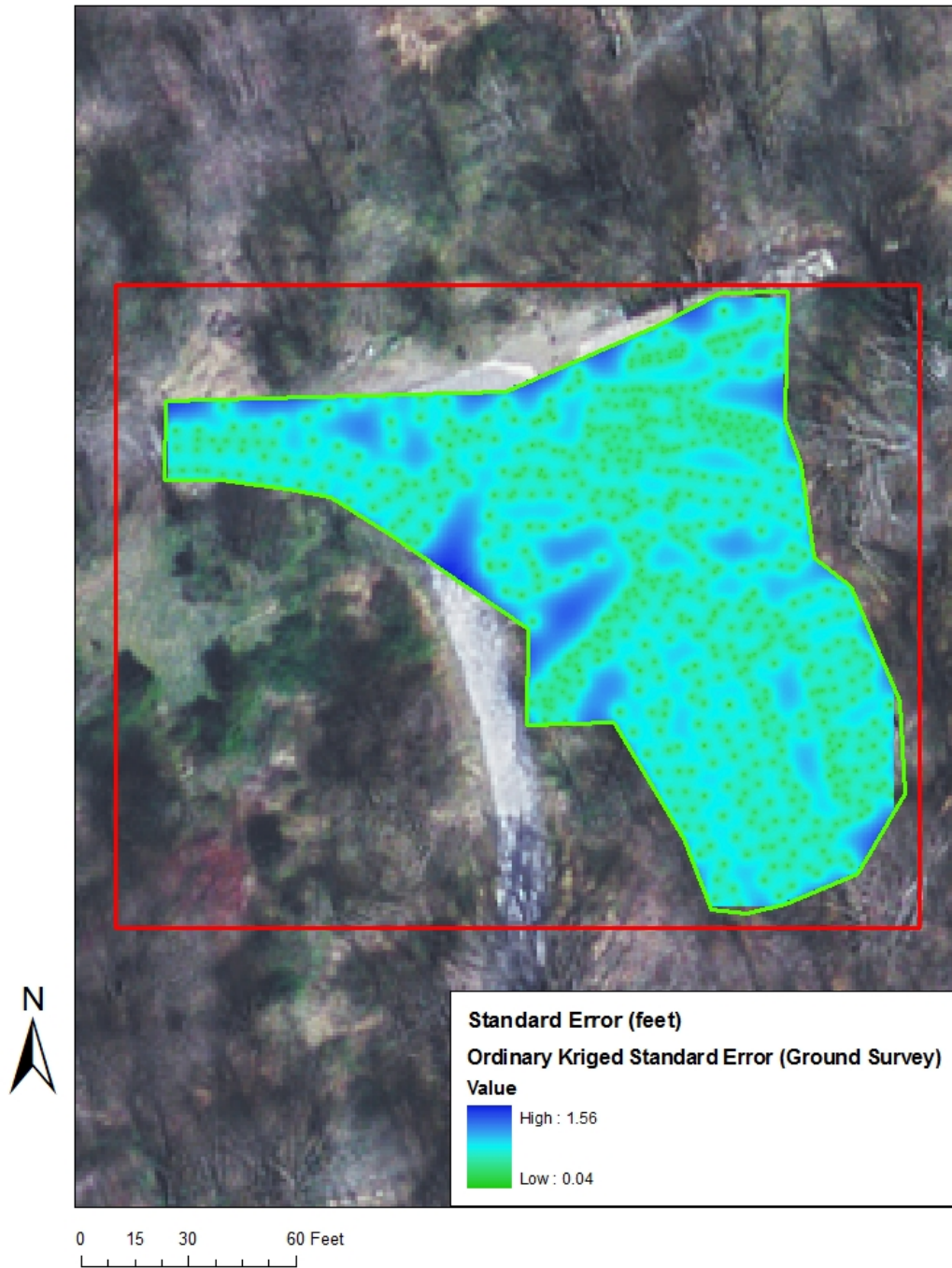
Figure 4-18. Ordinary Kriged Prediction Standard error raster created from the Kriged prediction standard error map using ground-surveyed points.
