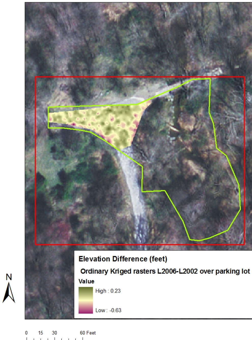
Figure 4-39. Parking Lot Difference of the Ordinary Kriged Prediction raster (LiDAR 2006 – LiDAR 2002). Mean Difference is -0.15298 feet which was used to adjust the LiDAR 2006 raster for systematic error.
