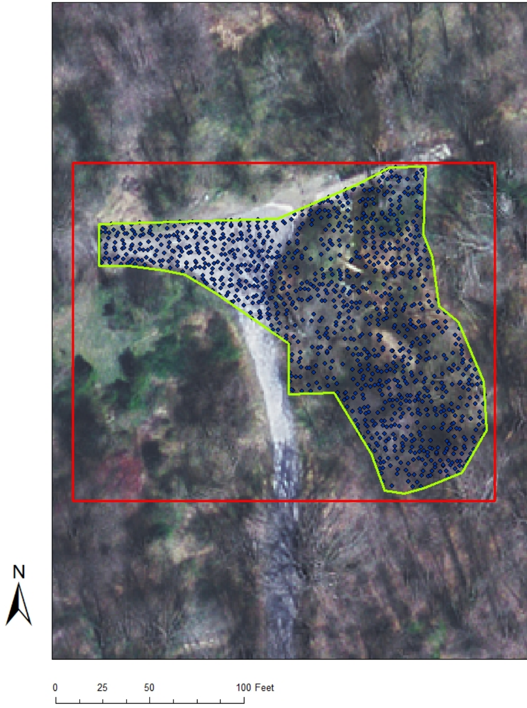
Figure 4-29. LiDAR 2002 points within the ground point polygon
