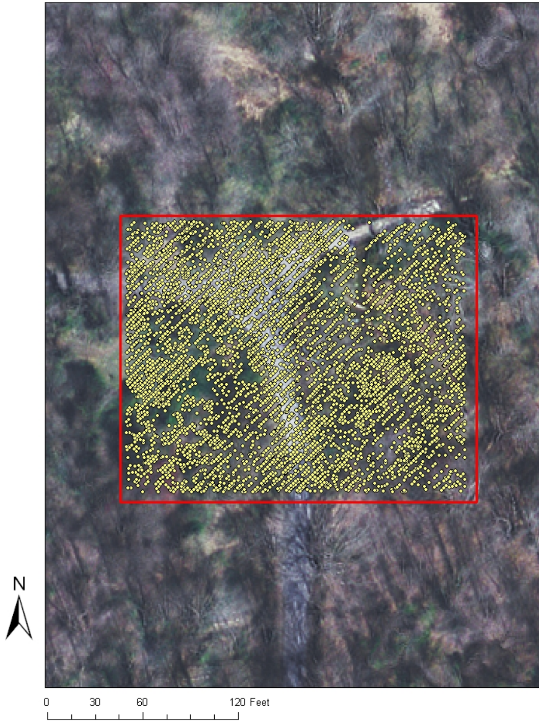
Figure 3-4. CSPA showing LiDAR 2006 point density (1.17 per square meter) within the AOI
