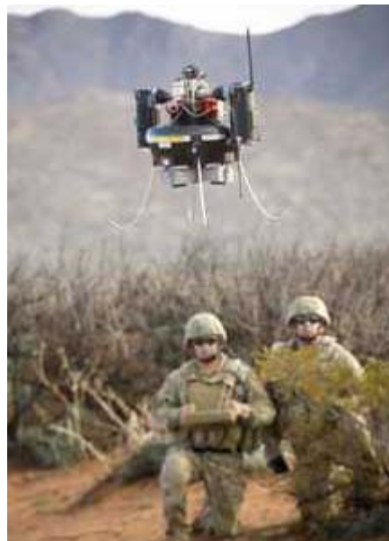
Figure 1.16: Honeywell Ducted Fan UAV model and demonstrated in active flight tests.
