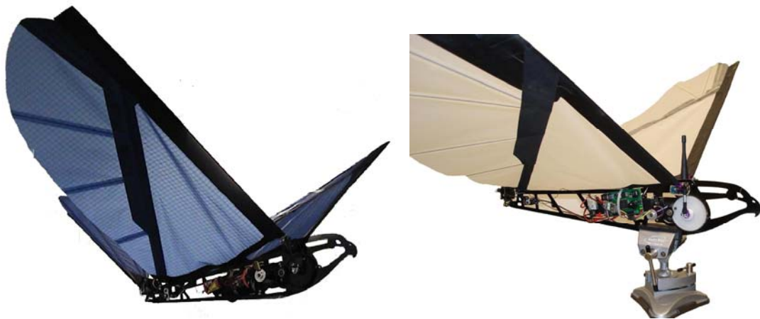
Figure 1.2: Blue ornithopter with 1.07m (42") span and white ornithopter with 1.22m (48") span.
