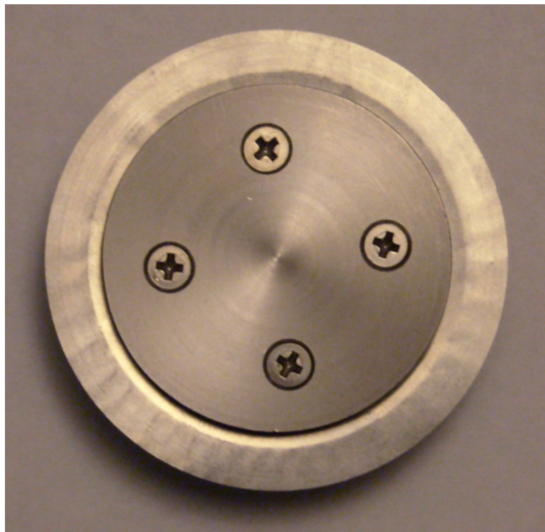
(a) Pump head assembly with discharge and intake reed ports
