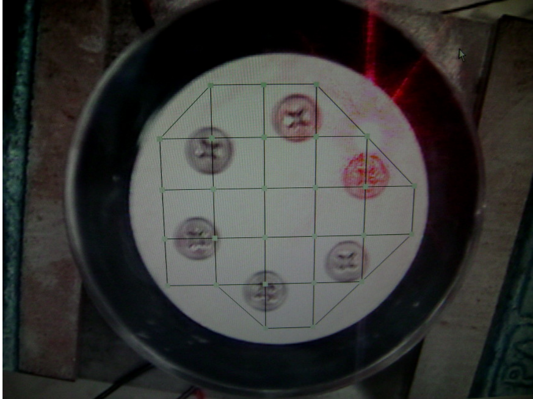
Figure 4.7: Scanning grid used for vibrometer measurements
