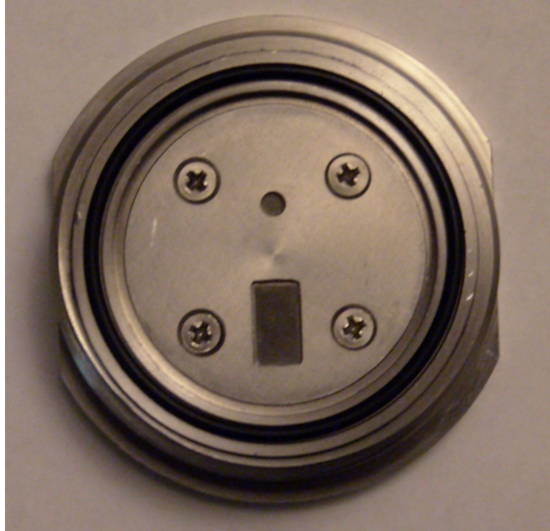
(a) Pump head assembly with discharge and intake reed ports
