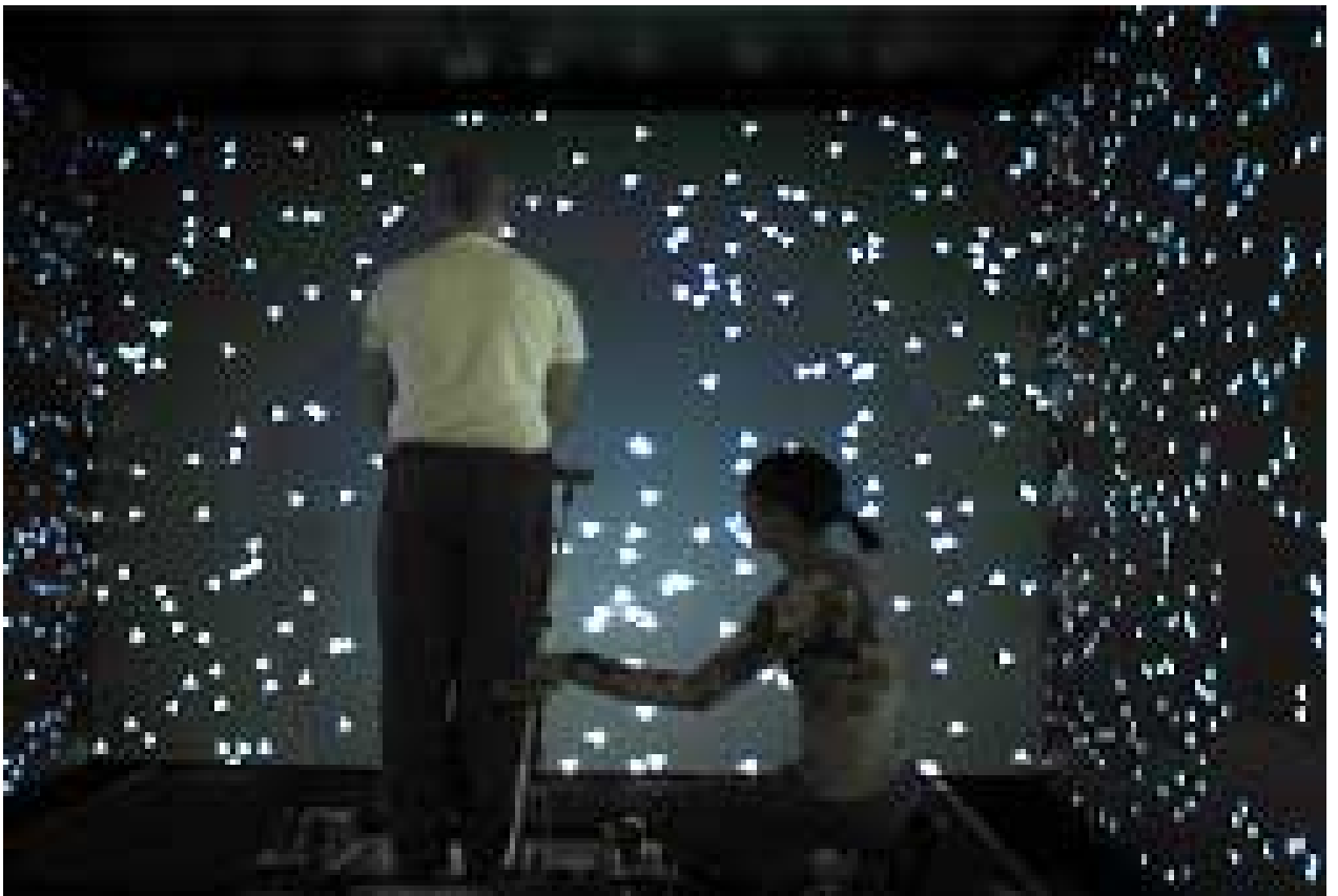
Figure 5 Visual virtual reality environment during a sway-referencing experiment.
