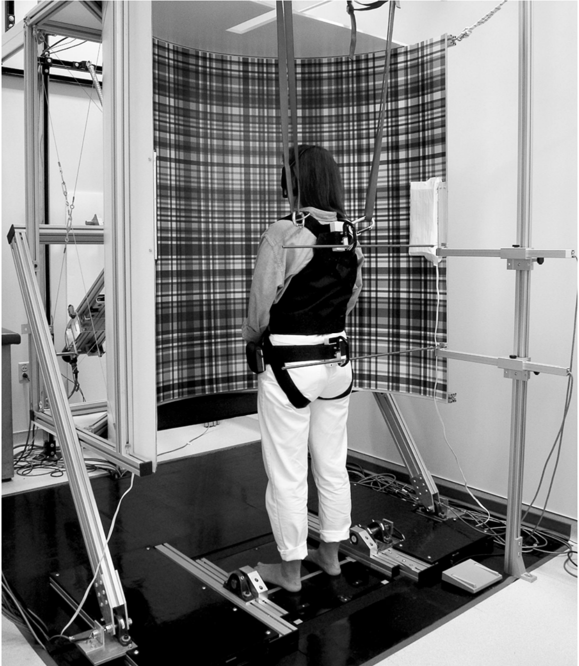
Figure 1. Experimental apparatus showing subjects standing on a sway-referenced platform.
