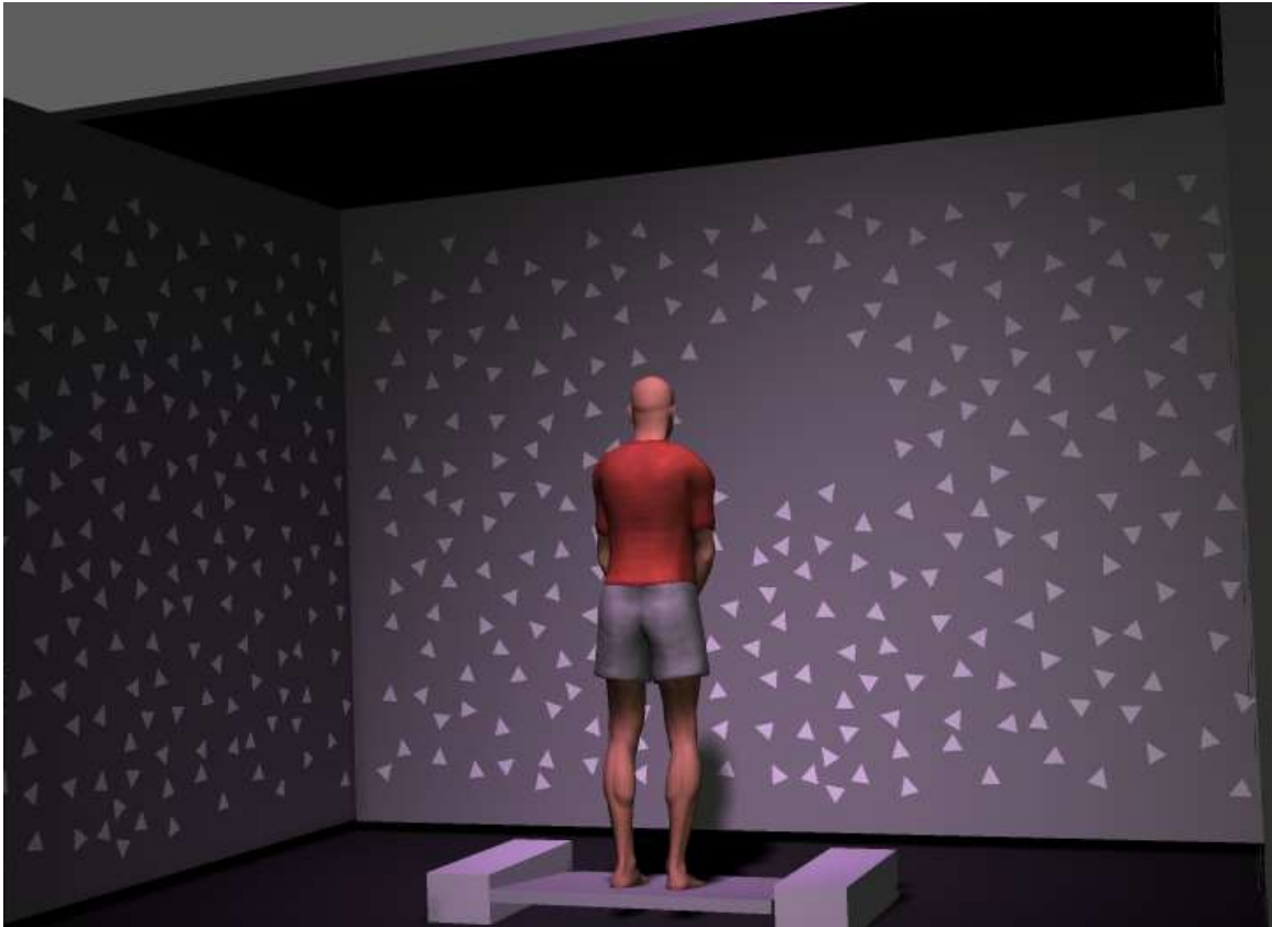
Figure 2. Virtual reality “cave” with sway-referencing platform.
