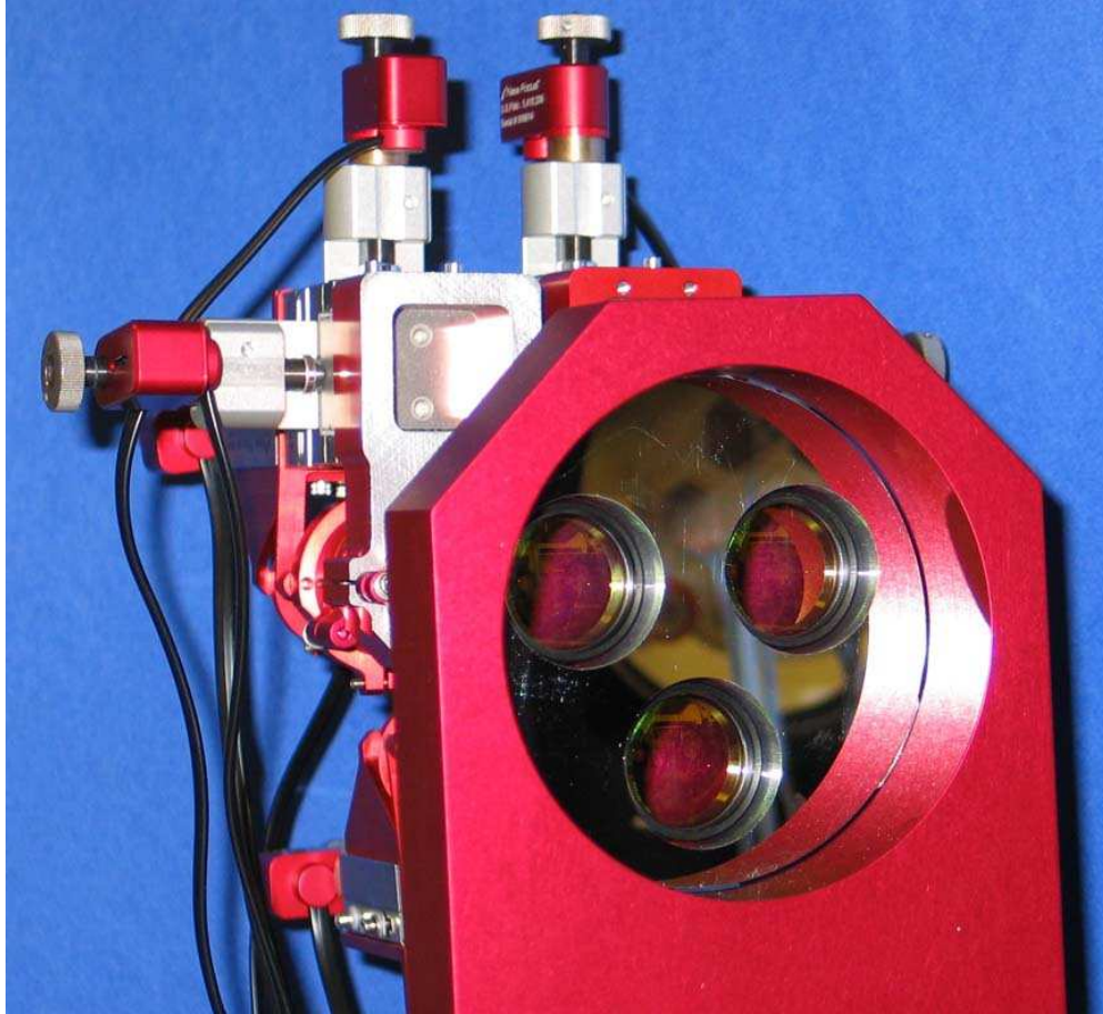
Figure 3.5: Conformal optical transmitter with three subaperture elements.
