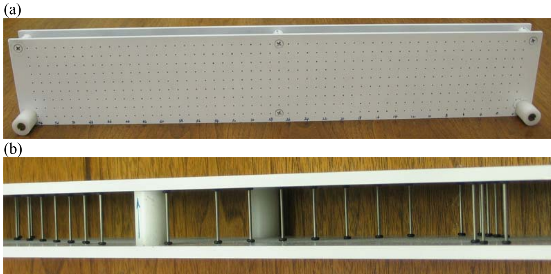
Figure 4.7 Photos of the calibration object: (a) side view; (b) top view with the steel pins inserted at known geometrical positions.
