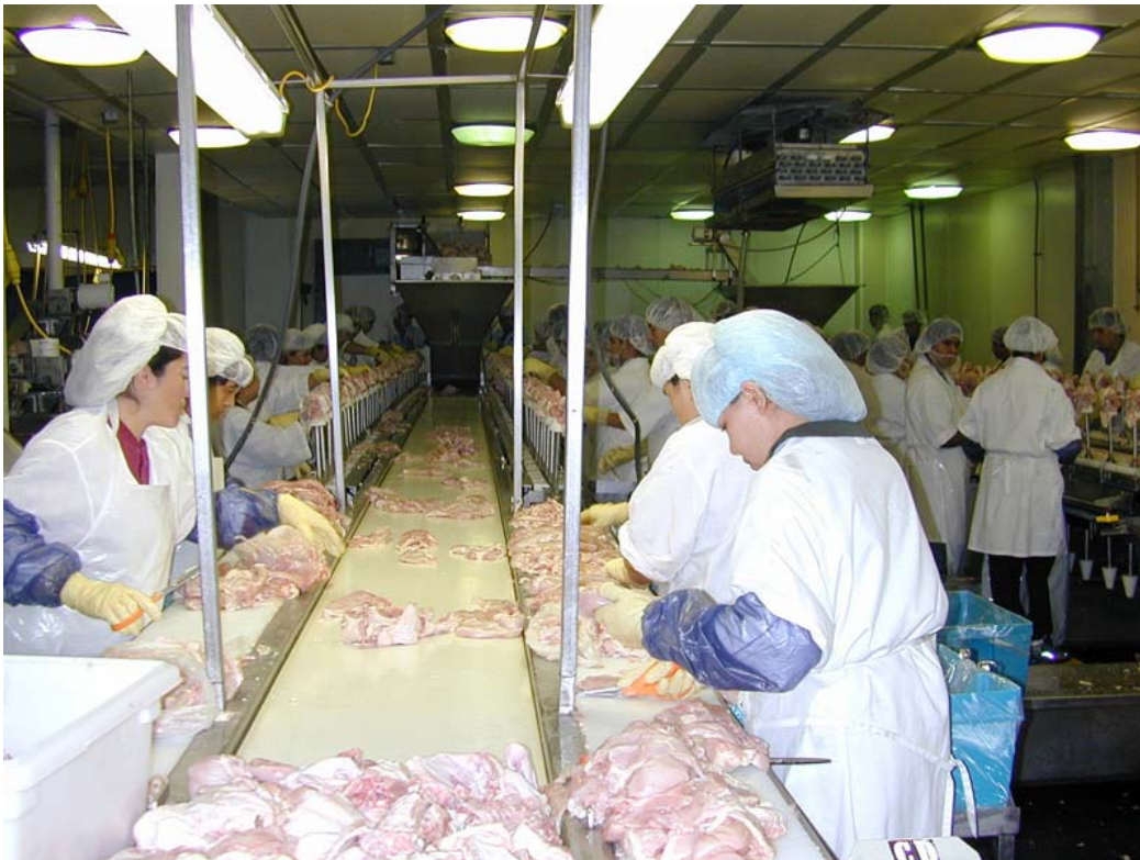
Figure 1.1 Poultry processing line. Note the physical contaminants inside meat are inspected manually by the workers.
