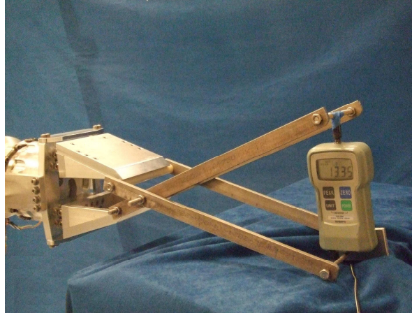
Figure 5.10: Force measurement test setup.
