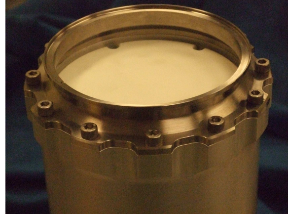
Figure 4.5: Manipulator link-flange interface.
