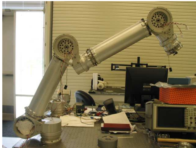
Figure 7.6: Image of the elbow pitch joint at maximum rotation.
