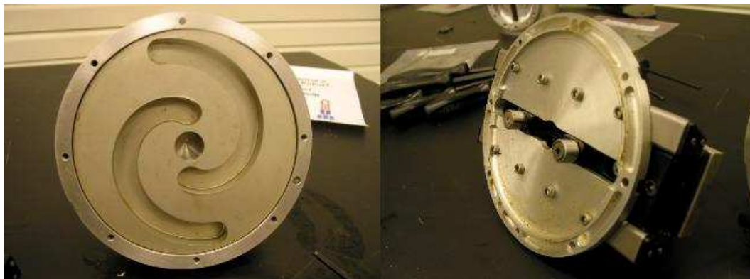
Figure 2.10: Ranger Spiral Plate (left) and Associated Track Rollers (right)
