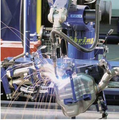
Figure 2.1: Welding torch end-effector (from [6]).
