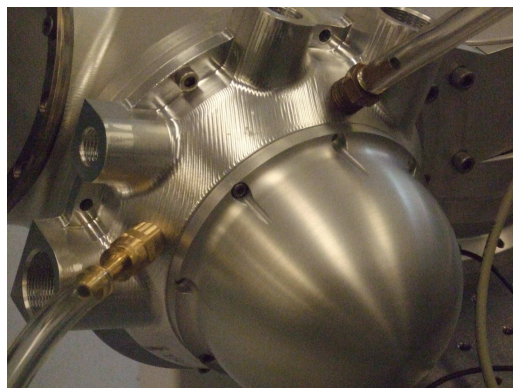
Figure 3.5: Oil hose barbs inserted in penetrator plate.
