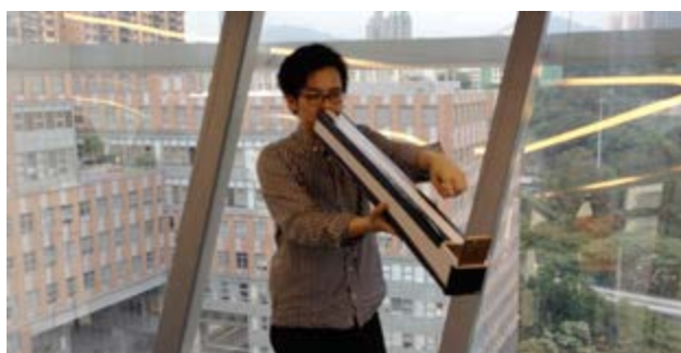
Figure 5. Sound periscope concept being demonstrated as an audio equivalent to the ubiquitous selfie stick.
