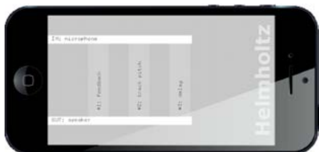
Figure 6. Helmholtz app. Each button routes the input (mic) to the output (speaker) in a different manner allowing feedback effects to be explored and mixed together (unaffected, pitch tracking and delay).
