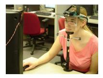
Figure 2.1: *Experimental setup for the user study with the ISCAN ETL-500 eye-tracker.* issues such as hypotheses, stimuli, and participants of the studies will be explained in Sections 2.4 and 2.5 in detail.
