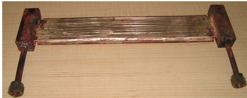
Figure 8: Copper microchannel heat exchanger for second generation TE Subcooler.
