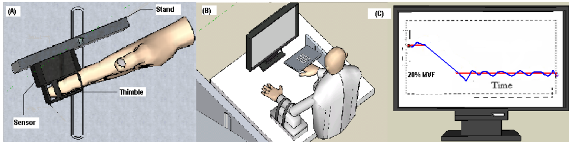
Figure 2.1. Experimental Setting: (a) The experimental setting for the right hand: the wrists and the forearm of the subject were rested in a wrist-forearm brace and held by Velcro strap. The subject sat in a chair and watched the computer screen to perform a task. (b) The subject inserted the distal phalange of each finger in the thimbles. The sensor positions were adjusted along the aluminum frame.(c) Subjects were asked to follow the template shown on the computer screen (red line), and given a feedback of their performance (blue line).
