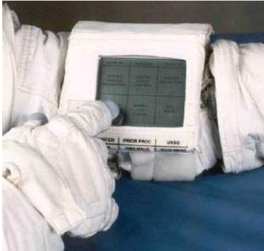
Figure 2.7: NASA's electronic cuff checklist prototype using a liquid crystal display and touch screen control interface. (courtesy of NASA )
