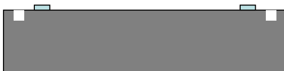
5) RIE and photoresist stripping
