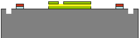
13) Photolithography for Al protection and Descum
