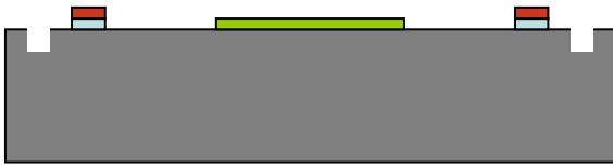
7) Photolithography for Al protection and Descum
