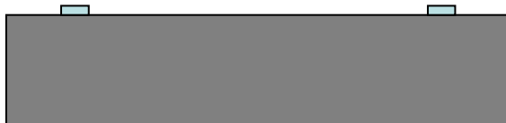
3) Al wet etching and photoresist stripping
