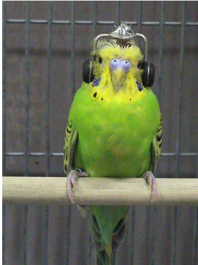
Figure 7. Image of a subject with a set of training earphones attached. Earphones were constructed of thin steel wire and rubber grommets and could easily be attached or removed from the animal. Refer to text for a complete description of earphone construction and attachment.
