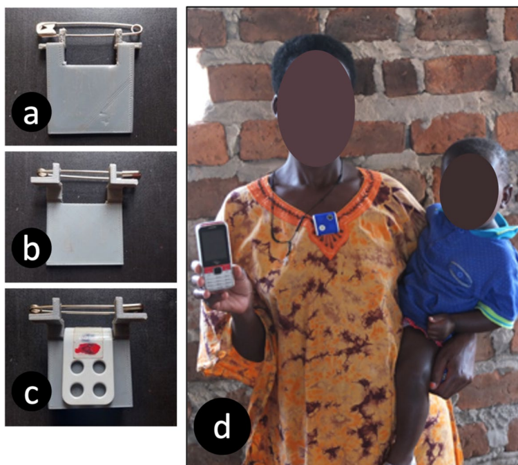
Fig. 2 The AWC affixed via a bespoke clip to the neckline of participants’ clothing
