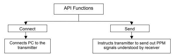
Two separate programs incorporating the provided API were written. The first program is meant for navigation of jumbo bird through keyboard inputs. The second program is an open loop program, meant for self-navigation of jumbo bird with time.
