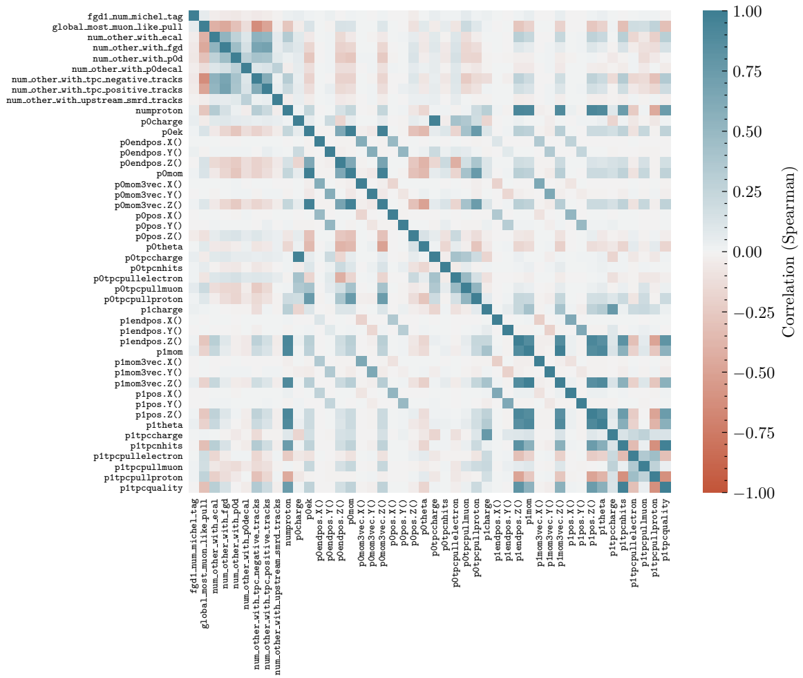
Fig. 7.7 Matrix of Spearman's rank pairwise correlations on the training dataset including all 46 reconstructed variables. Descriptions of these variables are given in Table 7.6.
