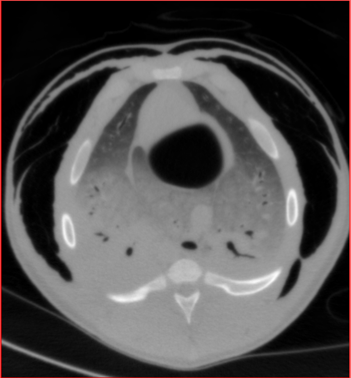
Figure 5.20 Image reconstructed using 7 iterations of OS-25 using 1498 \times 580 sinograms at 1024 \times 1024 pixels
