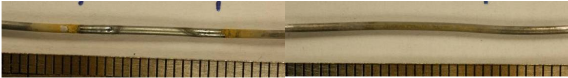
Figure 4.9: Galvanized 1006-1008 Carbon steel after 1 hour exposure to hydrogen (left) and methane (right). The scale markings are in mm. No flames are present.
