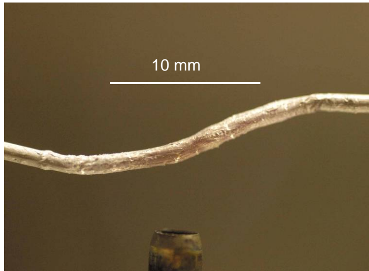
Figure 4.7: Color image of aluminum wire subjected to a hydrogen flame. Corrosion and severe deformation are observed. A hydrogen flame is present in this picture, but not visible.
