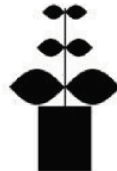
(d) Plant-shaped with 6 leaves patch antenna (2020, [92]), 1.12-10.02 THz (wide bandwidth, 159.78%), gain =18.66 dBi at 7.5 THz, and it is designed on polyamide substrate.
