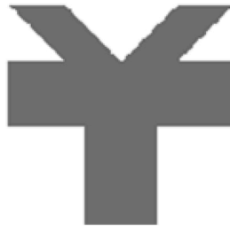
(b) Inverted K-shaped patch antenna (2020, [90]), 0.46-8.84 THz (very wide bandwidth), gain= 22.1 dB at 8.8 THz, radiation efficiency= 72 -93 %, and material used is perfect electrically conducting (PEC) on polyamide substrate.
