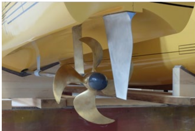
Fig. 8, A close-up view of the stern area with fitted propellers, shafts, brackets and rudders of the Stavanger demonstrator.
