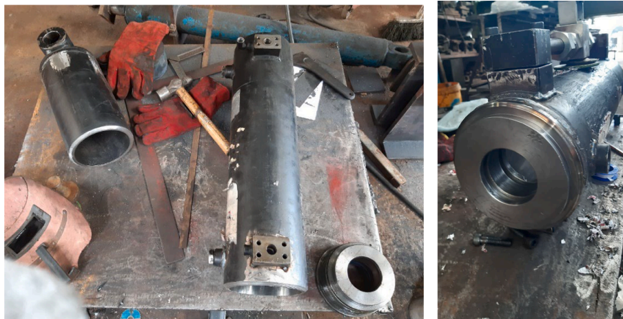
Fig. 10. Fabrication of the hydraulic cylinder of the SABFD device.
