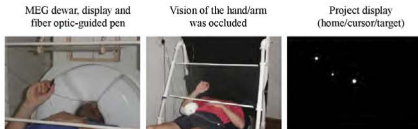
Fig. 1. Experimental setup. The subjects' view of their hands and arms has been occluded during the experiment. The participants were asked to move an optic pen on a plexiglass panel in front of them. A camera captured the movement of the pen tip and transformed it into cursor movement on a screen over the subjects' heads.
