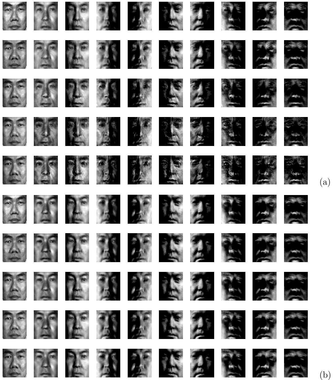
Figure 2.8: Image relighting/rendering results using (a) ISP-SLS and (b) multiple light source algorithms. For each row, the left image is the reference image used for estimating the surface normals and albedos and the remaining nine images are rendered ones corresponding to the nine lighting conditions in Eq. (2.21).
