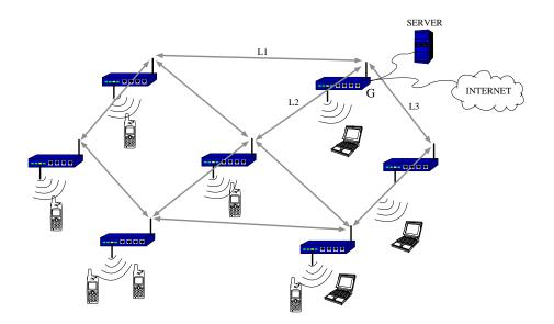
Figure 1.2: A typical wireless mesh network with a central authentication server.
