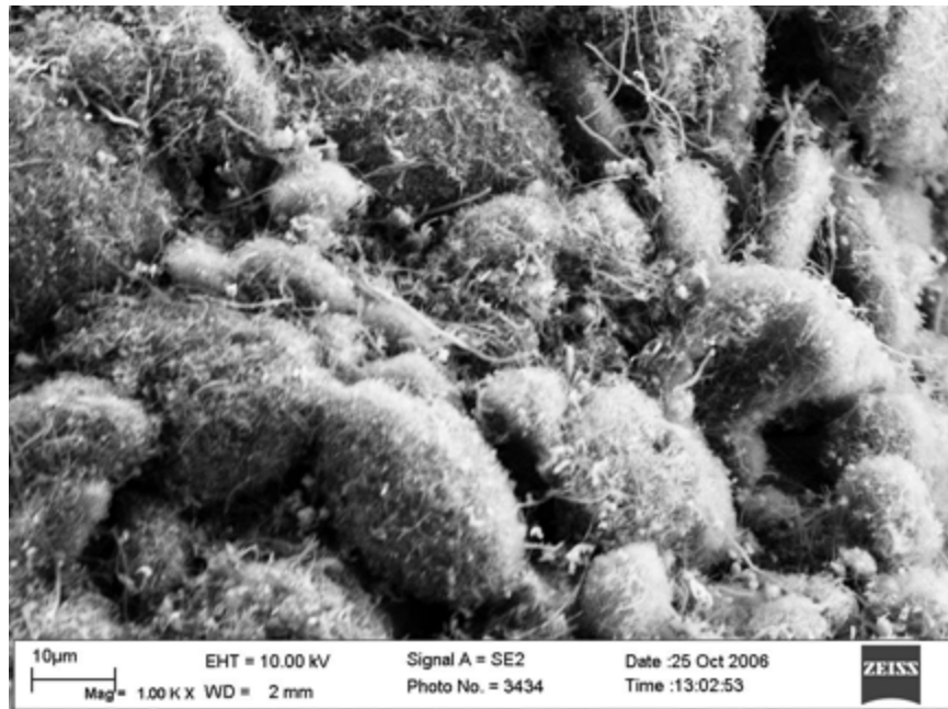
Figure 3.9 The as-received CNF agglomerates at a higher magnification.
