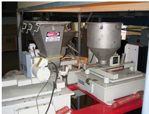
Figure 3.25 The loss-in-weight overhead feeders to feed powders and pellets.
