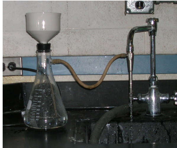
Figure 3.16 The vacuum filtration setup to separate the polymer nanocomposite precipitate after solvent extraction.
