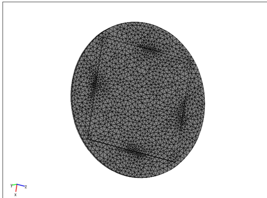
Figure 2.6: COMSOL mesh image dividing the system into small geometries in order to calculate stresses and strains of the window on the O-ring given 5 psi of pressure.
