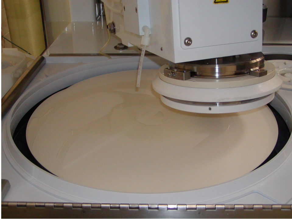
Figure 3.23. The polishing area of the Strasbaugh 6EC CMP tool. Polishing platen and pad, wafer carrier, polishing arm, and slurry dispenser can be seen. This tool has a 4” wafer chuck inside the wafer carrier.
