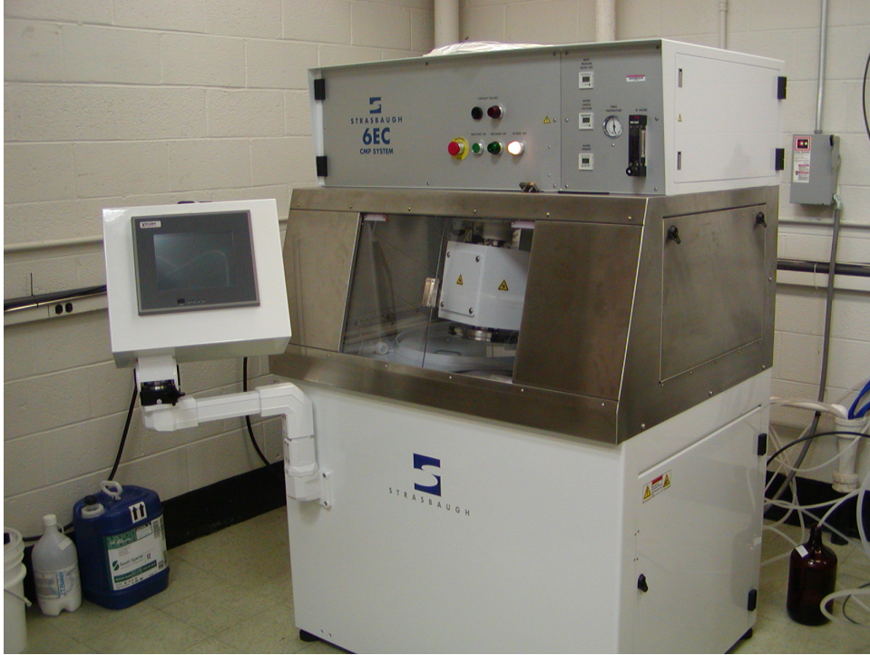
Figure 3.22. Strasbaugh 6EC CMP tool. The main unit, including polishing area, control panels, and touch-screen computer is shown.
