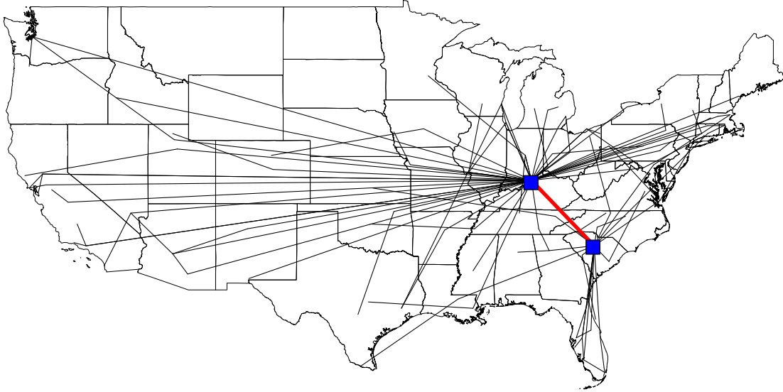
Figure 8.4: Optimized network configuration for two-stage operation (KY-SC, Q = 0.8M , u_i = 150,000 )
