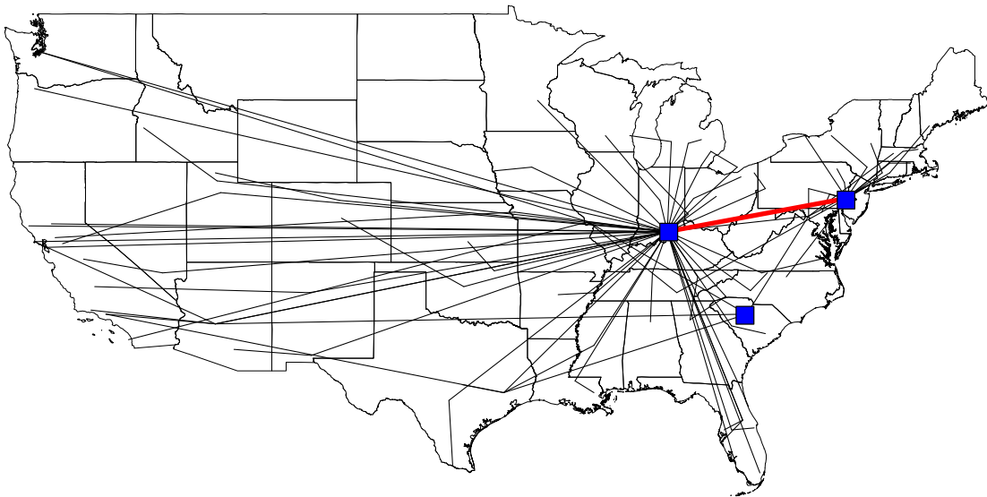
Figure 8.3: Optimized network configuration for two-stage operation (KY-PA, Q = 0.8\text{M} , u_i = 150,000 )
