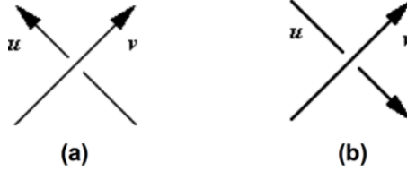
Figure 3.1: When projection of a pair of oriented line segments results in an overcrossing, its value is determined by the right-hand rule involving the projection direction and directions of projected line segments. Here the projection direction is from the page to the reader. (a) The value of this overcrossing is +1 because the bottom line segment ( u ) is in the counterclockwise direction from the upper line segment ( v ). (b) The value of this overcrossing is -1 because the bottom line segment ( u ) is in the clockwise direction from the upper line segment ( v ).
