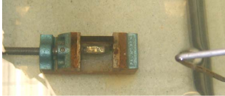
Figure 4.23 Packaged device held on the vice placed inside the water tank
