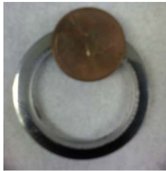
Figure 4.6 Nickel deposited on a polycarbonate substrate shaped in a ring structure
