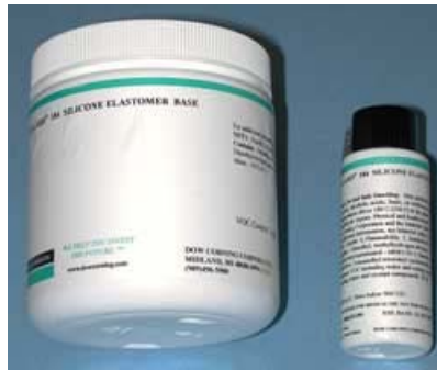
Figure 2.9 SYLGARD-184: two part silicone elastomer consisting of silicone resin and curing agent
