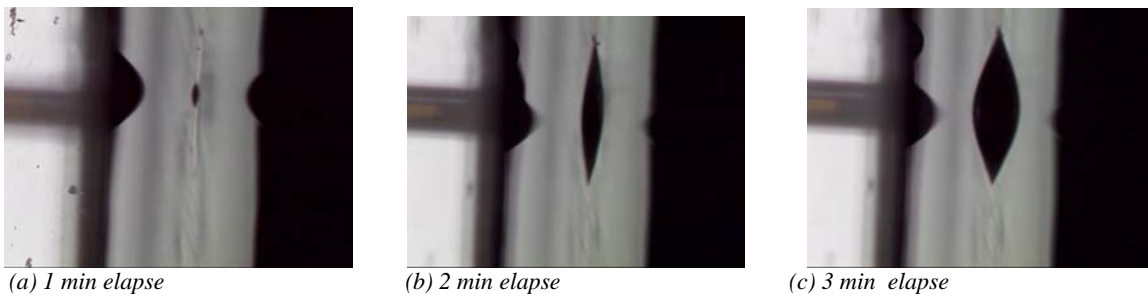
Figure 6-1 Taylor Cones Observed for 300 \mu\text{m} spacing with time elapsed, 2.1KV applied
