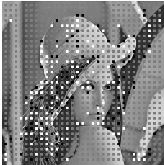
Figure 6.2: Illustration of better performing concealment schemes between GSB and OASI on the “Lena” image: OASI performs better (white blocks); GSB performs better (black blocks); GSB and OASI do not have significant performance difference (gray blocks).
