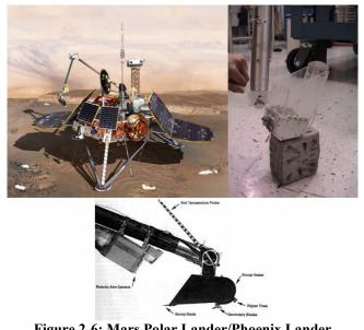
Figure 2-6: Mars Polar Lander/Phoenix Lander (Top L) Mars Phoenix Lander/Polar Lander Artist's Concept (NASA used same image for both probes) [19], (Top R) Phoenix Test Scoop [19], (Bottom) Mars Polar Lander Scoop [16]
