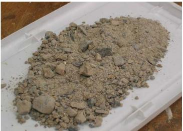
Figure 7-2: 210 g Sample of Soil Fines and Rock Fragments
