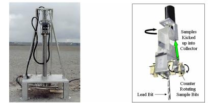
**Figure 2-11: Honeybee Robotics Sampling Systems** (*L*) *Mars Deep Drill (10 m), (R) Touch and Go Sampler [21]*
