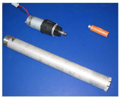
Figure 4-10: Drill, Bit, and Core Tube
