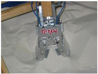
Figure 7-1: TERPS Collecting Pure Soil Sample
