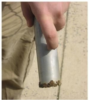
Figure 7-6: 4 cm Soil Core
