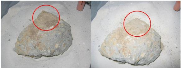
Figure 7-10: Before and After Rock Abrading
