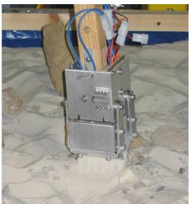
Figure 7-3: TERPS Sifting Soil Sample
