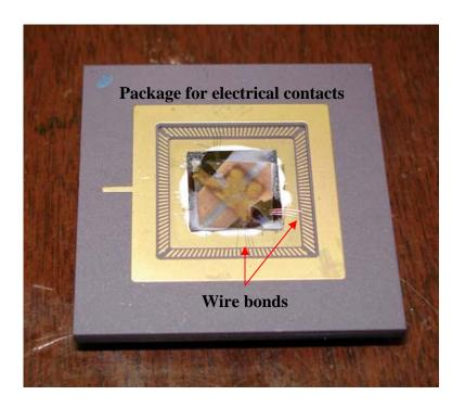
**Figure 4.13** – Digital photograph of the nanowire array based gas-sensing device glued to a package containing pin contacts for electrical connections.
