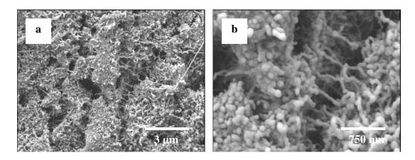
Figure 2.13 –  $SnO_2$  nanotube surface following  $SnO_2$  CVD and removal of CNT templates
