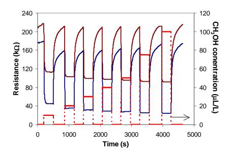
**Figure 2.15** – Typical gas sensing responses measured from a  $SnO_2$  nanotube covered microhotplate sample to varying concentrations of methanol (red, axis on the right) at 300 °C (brown, top) and 400 °C (blue, bottom).
