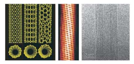
**Figure 2.1** – Schematic diagram of graphitic sheet structure of carbon nanotubes and a transmission electron microscope image of a multi-walled nanotube. Reproduced from Ref. [35].
