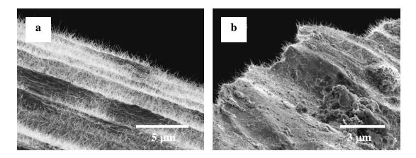
**Figure 3.7** – Nanowires grown on the surface of a commercial tungsten wire heated at 550 °C in RF  $Ar/H_2$  plasma. Some nanowires extend out from the edge of the wire.
