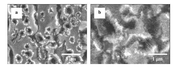
**Figure 2.12** – Vertically aligned CNT forests grown directly on a microhotplate. The nanotubes completely covered the sensor pads.
