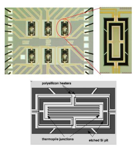
**Figure A1** – Optical images of a 6-element array of micro-calorimeters integrated on a chip and a closer look at an individual micro-calorimeter are shown on top. A schematic diagram of the device configuration is shown below.
