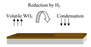
Figure 3.10 – Vapor-solid growth mechanism of WO<sub>x</sub> nanowires
