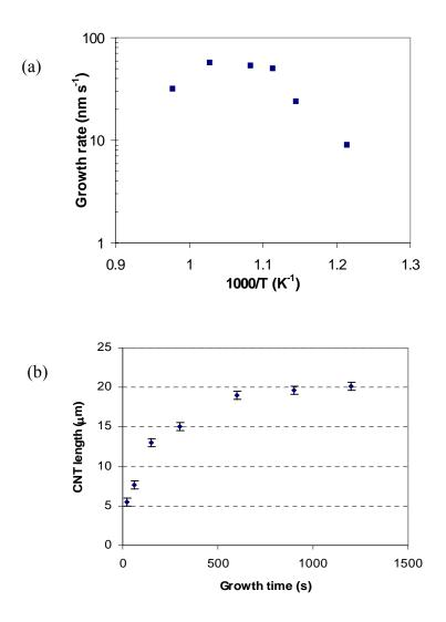
**Figure 2.10** – Influence of growth temperature (a) and growth time (b) on CNT array lengths. Temperature for growth time study =  $620 \degree$ C.
