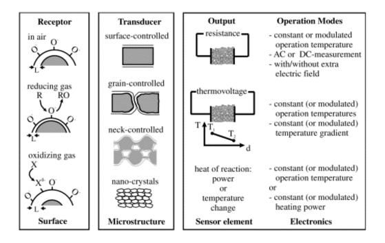
**Figure 1.2** – Schematic view of the physics of chemical gas-sensing devices. Reproduced from Ref [18].
