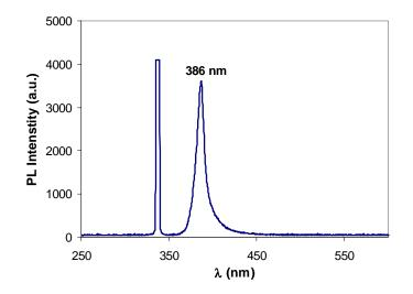
**Figure 4.6** – Room-temperature PL spectrum collected from Au catalyzed ZnO nanowire arrays on Si. The 338 nm peak corresponds to the exciting  $N_2$  ion laser while the 386 nm peak is recorded from the ZnO nanowires.
