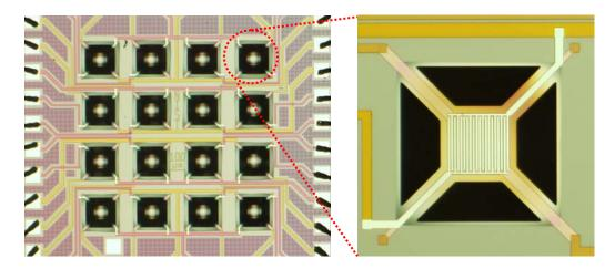
**Figure 2.11** – Optical images of a 16-element microhotplate array and a single microhotplate consisting of interdigitated comb-like contact pads (Distance between pads  $\approx 2 \ \mu m$ )
