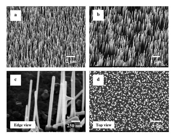
**Figure 4.3** – Aligned ZnO nanowire arrays grown on Au coated Si wafers at 550 °C. (a) and (b) were imaged from a  $45^{\circ}$  perspective.
