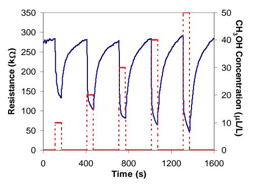
**Figure 4.15** – Sensor responses from the nanowire arrays at 325 °C to varying concentration of methanol (10 - 50 ppm).
