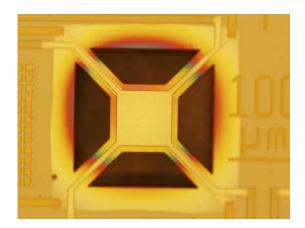
Figure 3.14 – Optical image of a tungsten thin film coated microhotplate device prior to nanowire growth
