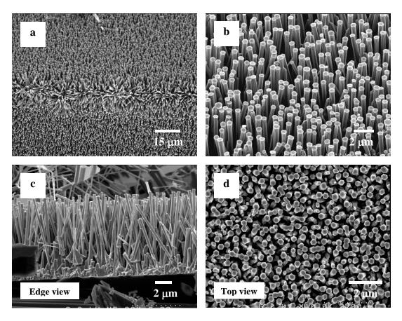
**Figure 4.2** – Aligned ZnO nanowire arrays grown directly on a Si wafer at 550 °C. (a) and (b) represent images of nanowires from a 45° perspective.
