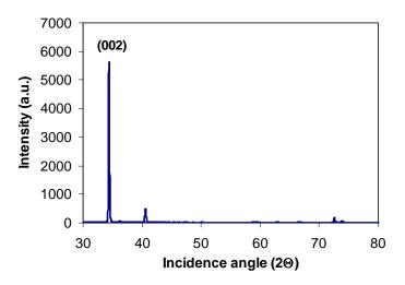
Figure 4.4 – XRD pattern of Au-catalyzed ZnO nanowire arrays grown on Si.
