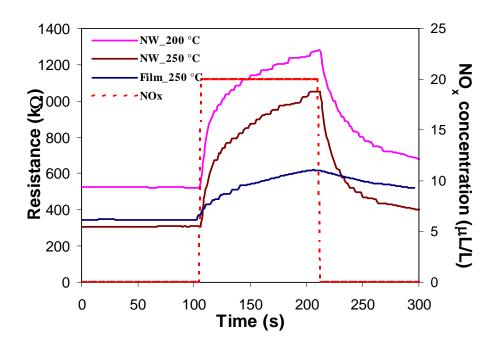
Figure 3.16 – Gas sensing responses to 20 ppm  $NO_x$  recorded from  $WO_3$  nanowires and a  $WO_3$  thin film
