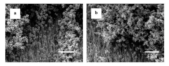
Figure 4.9 - SEM images of Ag nanoparticles resting above the ZnO nanowire array imaged from a  $45^{\circ}$  perspective.
