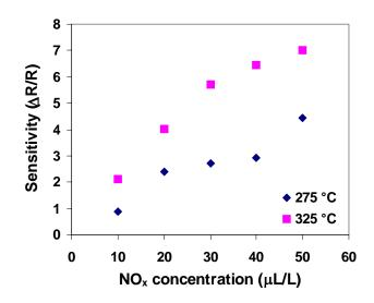
Figure 4.18 – Sensitivity of the nanowire array to nitrous oxide, evaluated at 275 and 325  $^{\circ}$ C.
