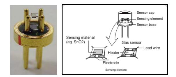
**Figure 1.3** – Digital photograph and schematic view of the components of a commercial Taguchi sensor. Reproduced from Ref [11].
