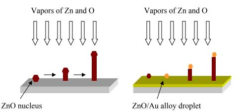
**Figure 4.7** – Non-catalytic V-S and catalytic VLS growth mechanisms of ZnO nanowires grown by chemical vapor transport.
