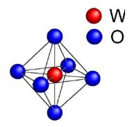
Figure 3.1 – Crystal structure of WO<sub>3</sub>
