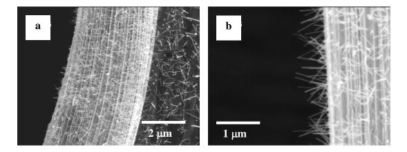
**Figure 3.8** – Nanowires grown on the surface of tungsten TEM grids heated at 550 °C in RF  $Ar/H_2$  plasma.
