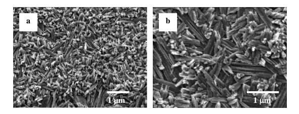
**Figure 3.3** – SEM images of grainy, nodular surface of tungsten film heat treated at 750 °C in pure Ar.
