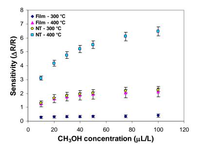
**Figure 2.16** – Sensitivity plots of microhotplate surfaces covered with  $SnO_2$  nanotubes (NT) and bare  $SnO_2$  thin films at 300 and 400 °C to varying concentrations of methanol.
