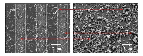
**Figure 2.6** – SEM images of microhotplate surface before and after  $SnO_2$  deposition. The arrows indicate specific shapes on the surface that were imaged to verify conformal coating.
