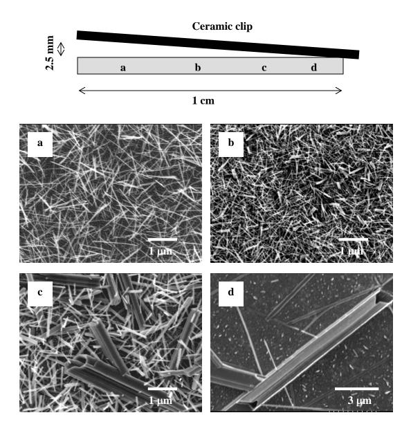
**Figure 3.11** – Schematic illustration of clip-substrate assembly used for mass-transfer dependence study. SEM images depict nanostructures grown in the regions indicated along the length of the substrate. (From left edge, a = 2 mm, b = 6 mm, c = 8.5 mm, d = 9.5 mm)
