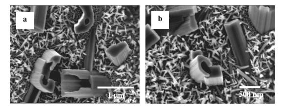
**Figure 3.13** – Irregular hollow nanostructures and solid nanorods observed to grow on a tungsten surface heated to 550  $^{\circ}$ C in RF Ar/CO plasma.
