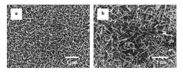
**Figure 3.12** – Uniform network of nanowires grown by heating a tungsten film to 550 °C in RF Ar/CO plasma.
