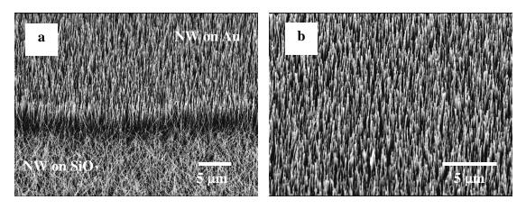
**Figure 4.11** – SEM images of gas sensing device sample surface. Vertically aligned nanowire grew on Au catalyst pads while randomly oriented nanowires grew on  $SiO_2$
