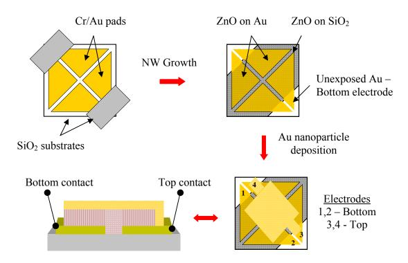
Figure 4.10 – Schematic diagram of gas sensing device fabrication steps. The bottom images represent side and top views of the device.
