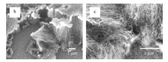
**Figure A2** – SEM images of CNTs grown on a micro-calorimeter device. (b) and (c) represent CNT forests grown on the sample zone.
