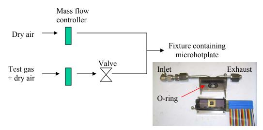
Figure 2.14 – Schematic representation of gas-sensing measurement setup
