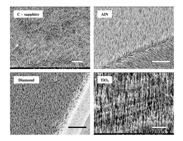
Figure A4 – Epitaxial growth of ZnO nanowires on various substrates. Scale bars represent 5  $\mu$ m.
