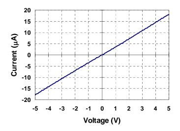
Figure 4.14 – I-V characteristic of the device following repeated heat treatments at temperatures up to  $350 \,^{\circ}$ C.
