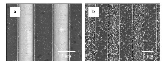
**Figure 2.5** – SEM images of microhotplate surface following (a) 30 nm sized Ni nanoparticle deposition; (b) carbon nanotube growth
