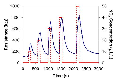
**Figure 4.16** – Sensor responses from the nanowire arrays at 325 °C to varying concentration of nitrous oxide (10 - 50 ppm).
