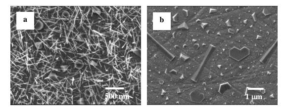
**Figure 3.5** – (a) Nanowires and crystallite structures grown by heat treatment of tungsten film at 600 °C in RF Ar/H<sub>2</sub> plasma. (b) Solid nanorods and other crystallite structures grown at 650 °C in RF Ar/H<sub>2</sub> plasma.
