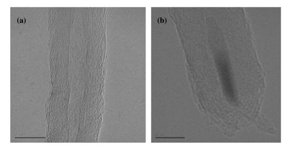
**Figure 2.9** – High-resolution TEM images of a single multi-walled CNT (grown on Au) clearly represent highly crystalline graphene sheets overlapping a hollow core. An oblong catalyst particle could be found on the tips of a few CNTs. The scale bars represent 10 nm.
