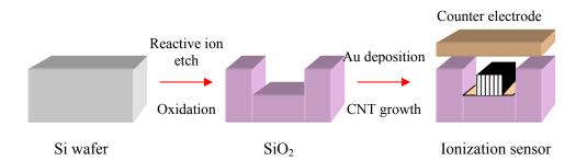
**Figure A3** – Schematic of steps involved in fabrication of CNT-array based gas-ionization sensor. Both trench depth and CNT lengths can be controlled to precisely adjust interelectrode gap through this approach.
