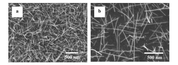
**Figure 3.4** – Uniform network of nanowires grown by heating a tungsten film at 550 °C in RF  $Ar/H_2$  plasma.
