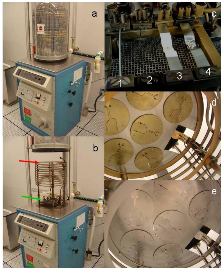
Figure 59: Metal evaporation steps in pictures. (a) The CVC thermal evaporator, (b) Evaporator with bell jar open to reveal metal source boats (green arrow) and target area (red arrow) where the PC wafer holder sits, (c) Close-up of deposition metals, (d) Wafer holder pre-evaporation looking up inside the evaporator, and (e) Wafer holder post-evaporation.
