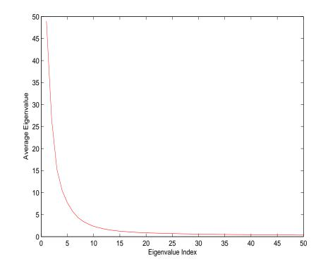
Figure 8.4: This plot shows the average eigenvalues for an anomaly detector using KPCA. It is easy to see that the eigenvalues die out very quickly. Results indicate that using the m most significant eigenvectors (where the corresponding m eigenvalues represent a large portion of the total energy in the eigenvalues) yield acceptable performance levels.
