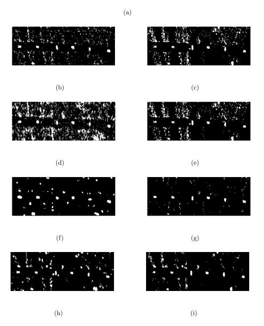
Figure 9.6: (a) Ground truth for the DR-II HYDICE image. Output results at 80% detection rate using (b) RX, (c) PCA, (d) FLD, (e) EST, (f) KRX, (g) KPCA, (h) KFD, and (i) KEST.
