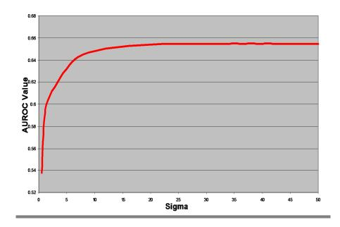
Figure 8.2: This figure shows an example of how  $\sigma$  was chosen in this thesis. The graph plots the area under the ROC (AUROC) curve as a function of  $\sigma$ . The value of  $\sigma$  corresponding to the greatest AUROC value was chosen as the kernel parameter. This example comes from a KEST analysis on the DR-II HYDICE image. Here, the optimal value for the kernel parameter occurs at around  $\sigma = 38$ .
