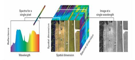
Figure 2.2: This figure shows the basic layout of a hyperspectral cube (center). The cube can be viewed in two ways. The first (left) is as a set of material spectra, one at each pixel location. The second (right) is as a spatial distribution of radiance (reflectance) data at one specific wavelength. Both ways are equally informative. [8]
