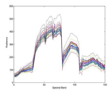
Figure 2.3: This image illustrates the spectral variability that is inherent in hyperspectral imagery. Shown here are 36 contiguous spectral signatures from a hypothetically homogenous background clutter region. All spectral vectors have the same basic shape yet none has an identical spectral signature.
