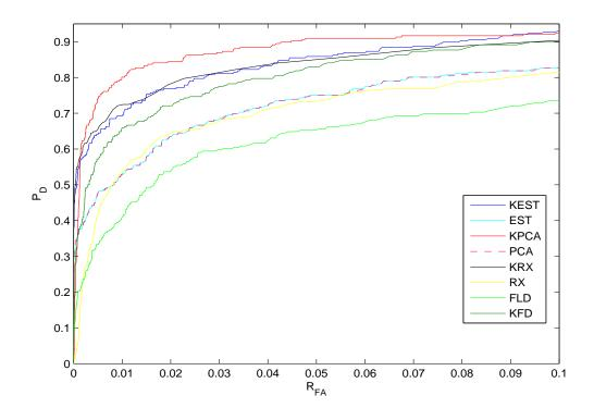
Figure 9.8: ROC curves for the DR-II image at very low false alarm rates.
