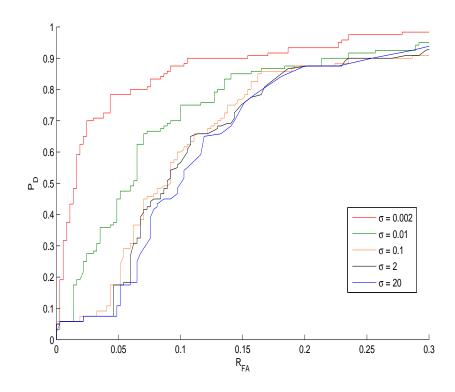
Figure 8.1: This figure illustrates the importance of choosing a good value of the kernel parameter,  $\sigma$ . Using  $\sigma$  values of [0.002, 0.01, 0.1, 2, 20], the detector performance changes drastically. If a bad value of  $\sigma$  was chosen, the detector would not perform up to its potential.
