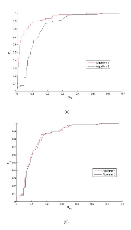
Figure 9.3: This figure illustrates the occasional difficulty in analyzing ROC curves simply by visual observation. In (a), it is quite clear that Algorithm 1 performs better than Algorithm 2. However, (b) illustrates a case where it is not so obvious which algorithm is best. The ROC curves here are extremely close and cross each other many times over the whole range of  $R_{FA}$ . This issue illustrates the need for the use of AUROC analysis.
