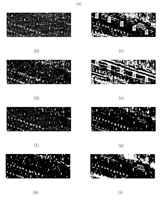
Figure 9.18: (a) Ground truth for the AHI-2 image. Output results at 80% detection rate using (b) RX, (c) PCA, (d) FLD, (e) EST, (f) KRX, (g) KPCA, (h) KFD, and (i) KEST.
