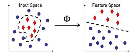
Figure 5.1: This figure displays the basic idea behind the use of kernels. In the input space, only a highly nonlinear decision boundary can be found to separate the data. However, if the data is mapped into a higher-dimensional feature space using  $\Phi$ , a linear separating hyperplane can (often) be found. By using kernel functions, it is possible to find this separating hyperplane without actually mapping the data into the feature space.
