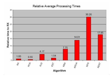
Figure 9.25: Relative implementation times per pixel for all eight methods on the HYDICE images. Each spectral vector is of length 150. All times are relative to the average processing time for the RX-algorithm.
