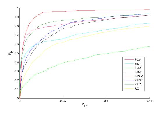
Figure 9.11: ROC curves for the FR-I image at very low false alarm rates.
