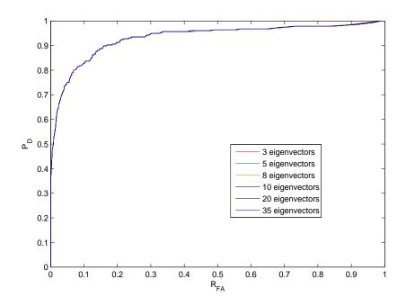
Figure 8.3: This figure shows an example of how the detector performance does not change significantly if the number of eigenvectors used as the bases vectors to generate the subspace is altered.
