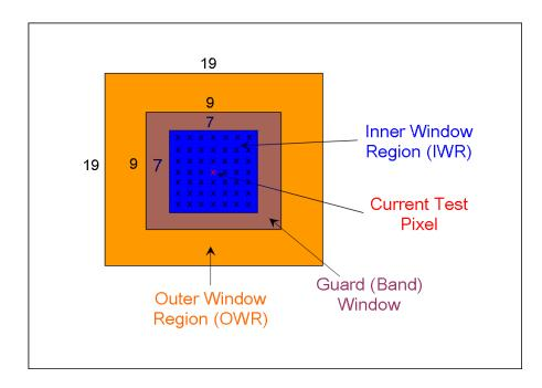
Figure 3.1: An example of a dual window with guard band. The numbers represent the length in pixels making up the side of each window. Each 'x' in the IWR represents one pixel. The pixel in red represents the current test pixel. The figure is not necessarily drawn to scale
