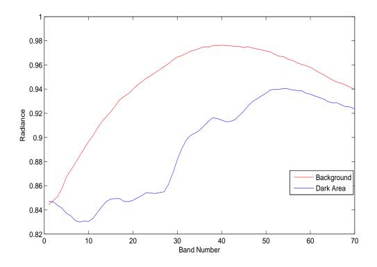
Figure 9.16: Average spectrum of background pixels versus average spectrum of dark area pixels in the AHI-1 image. The extreme difference in statistical properties between these two averages explains the high number of false alarms generated in this region.
