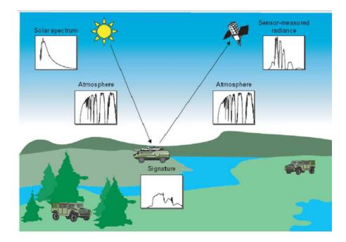
Figure 2.1: This figure illustrates the process involved in a hyperspectral remote sensing system. The spectrum eventually collected by the sensor is a combination of the solar spectrum, atmospheric attenuation, and the material spectral signature. [8]
