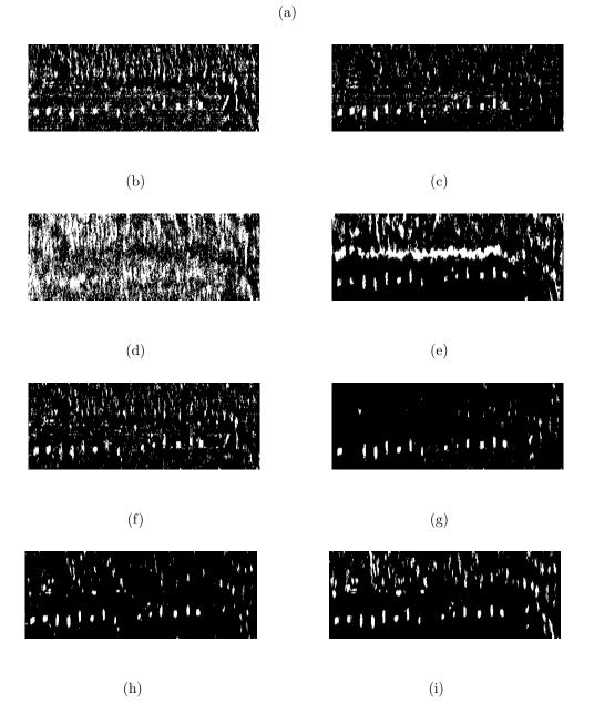
Figure 9.9: (a) Ground truth for the FR-I HYDICE image. Output results at 80% detection rate using (b) RX, (c) PCA, (d) FLD, (e) EST, (f) KRX, (g) KPCA, (h) KFD, and (i) KEST.
