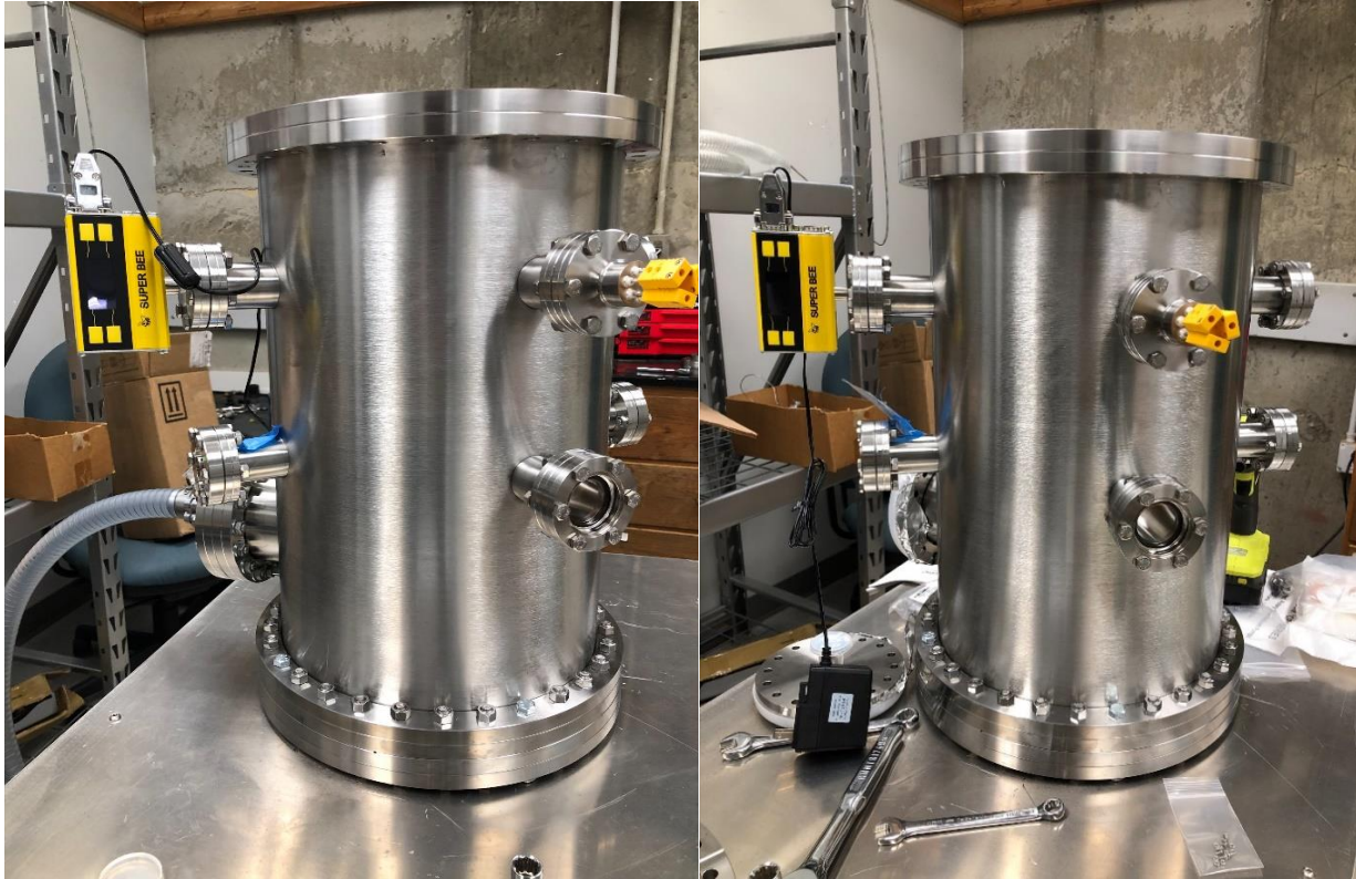
Fig. 5.3: Pictures of the Outer Solar System Astrophysics Lab at the Keck Laboratory for Planetary Simulations at the University of Arkansas. A CH-110LT 40K Cryocooler Series helium refrigerator system is attached to the chamber with the bottom flange adapter. The chamber has eight CF ports, of which 4 are fixed feed-thru and the rest 4 are rotating feed-thru. A pressure gauge is connected to the chamber with a feed-thru (see Super Bee pressure gauge attached on the left side of the chamber). For measurement of temperature inside the chamber, a thermocouple feed-thru is also connected to the chamber. For a higher resolution version of the diagram, the readers are referred to the online version of the figure.
