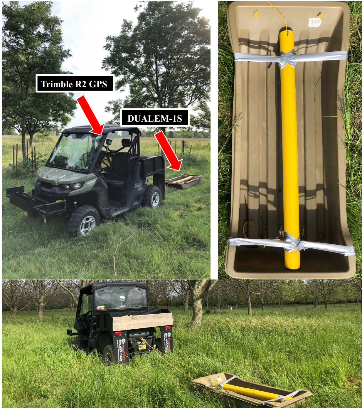
Figure 2. The survey setup included a DUALEM-1S sensor that was suspended on a sled that was tied to a Side-by-Side vehicle, a Trimble R2 global positioning system unit mounted inside of the Side-by-Side, and both the DUALEM-1S and Trimble R2 were connected to a Trimble Yuma 2 field computer inside the Side-by-Side that interpolated the data in a hand-held geoinformation system.
