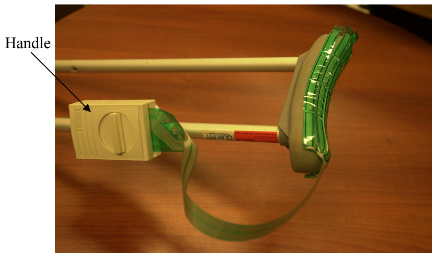
Figure 4.3: Axillary crutch with an Fscan sensor connected to the handle.
