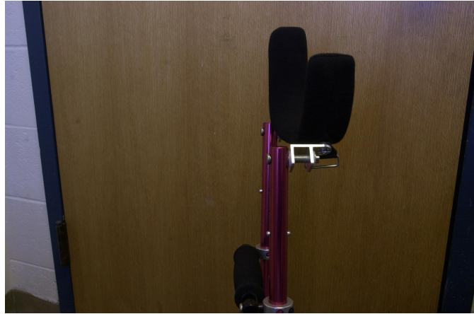
Figure 3.1: The shoulder support of the mini-Strutter is cantilevered on the red vertical support tube.
