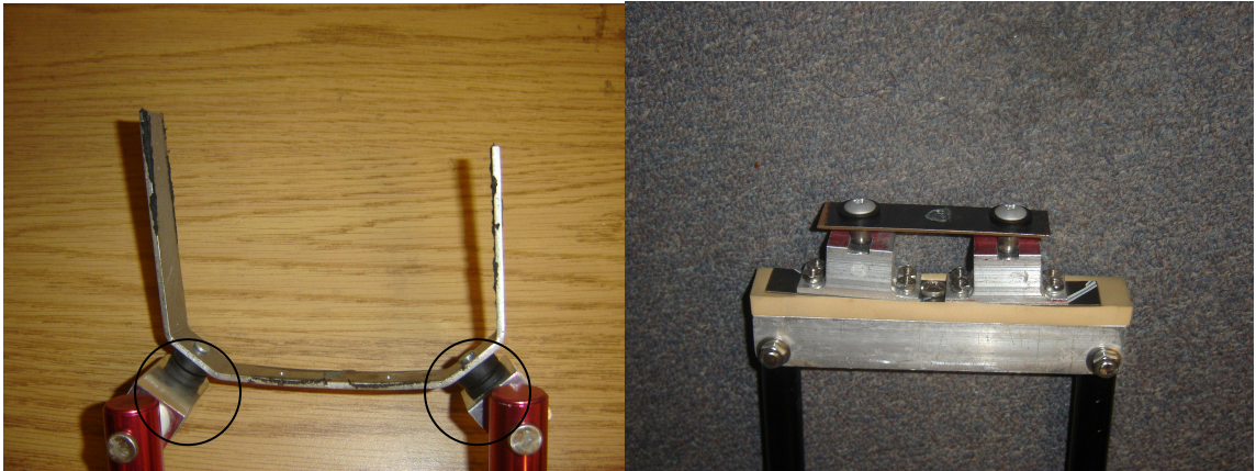
(a) (b) Figure 6.3: Shock absorbing gasket circled on the mini-Strutter (a) and prototype with shock absorbing axillary support (shock absorber is yellow and there are also dampers in the two boxes) (b).
