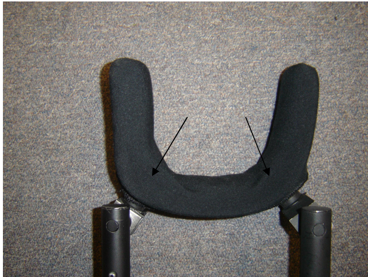
Figure 4.9: Location where the tape holding the sensor onto the axillary pad typically breaks free and folds.
