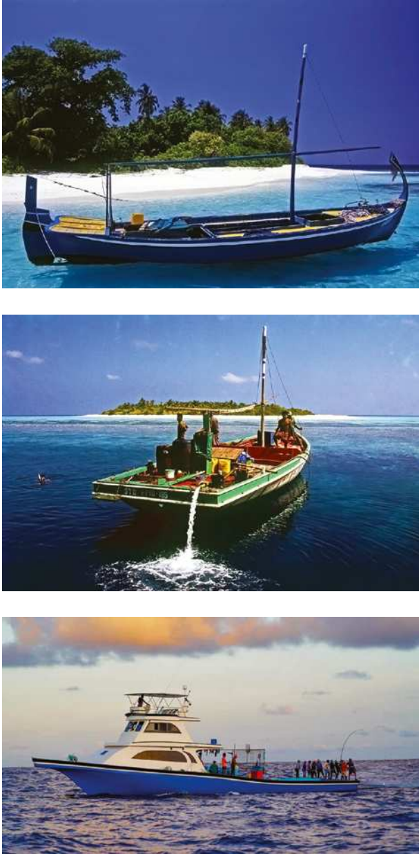
FIGURE 2 Types of fishing vessels a. Traditional mas dhoni b. Second generation mas dhoni with transom aft c. Third generation mas dhoni with accommodation SOURCE: A, B—MOOSA ISMAIL, MALDIVES, C—COURTESY 'ZUVAAN MASVERIYA'
