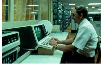
Figure 3.4. Univac 1108 mainframe console. Note 12" tape reels in background. Contents of about 3,000 such reels can now fit on a single 150GB 3.5" disk.
