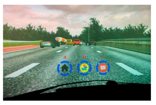
**Figure 3.** Three main interface symbols as appear in the VR driving simulator: (**a**) Home, (**b**) Navigation/Map, and (**c**) Text Message symbols.
