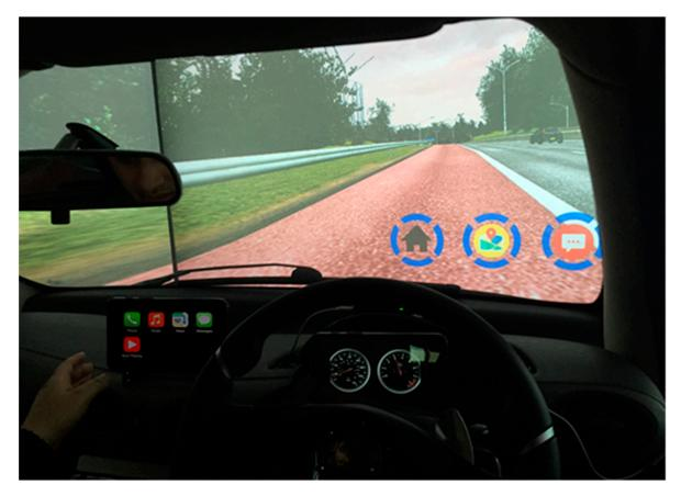
**Figure 1.** Screenshot of the fully functional Augmented Reality (AR) Head-Up Display (HUD) and conventional Head-Down Display (HDD) interfaces in the Virtual Reality (VR) driving simulator.
