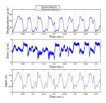
Figure 19: Experimental results of trajectory tracking using inverse control based on the dynamic hysteresis model.
