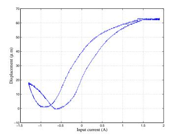
Figure 2: Hysteresis in a magnetostrictive actuator.
