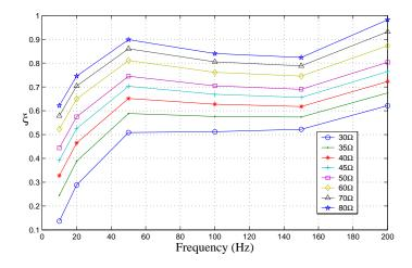
Figure 17: Identification of  $R_{eddy}$  and  $\xi$ .
