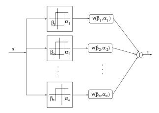
Figure 6: The discretized Preisach operator.
