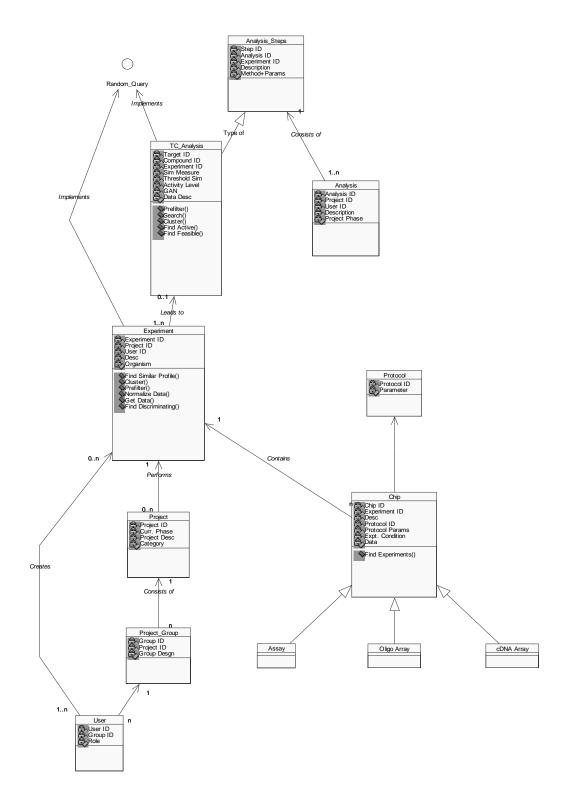
Fig. 4.11 Experiment and Administration Subsystem Class Diagram
