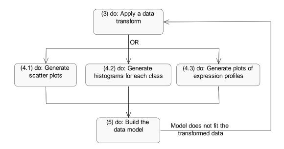
Fig. 4.15 Lower-level FFBD for Function 4: Generate Visualizations
