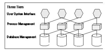
Fig. 4.19 Three-tier Client/Server Architecture [37]
