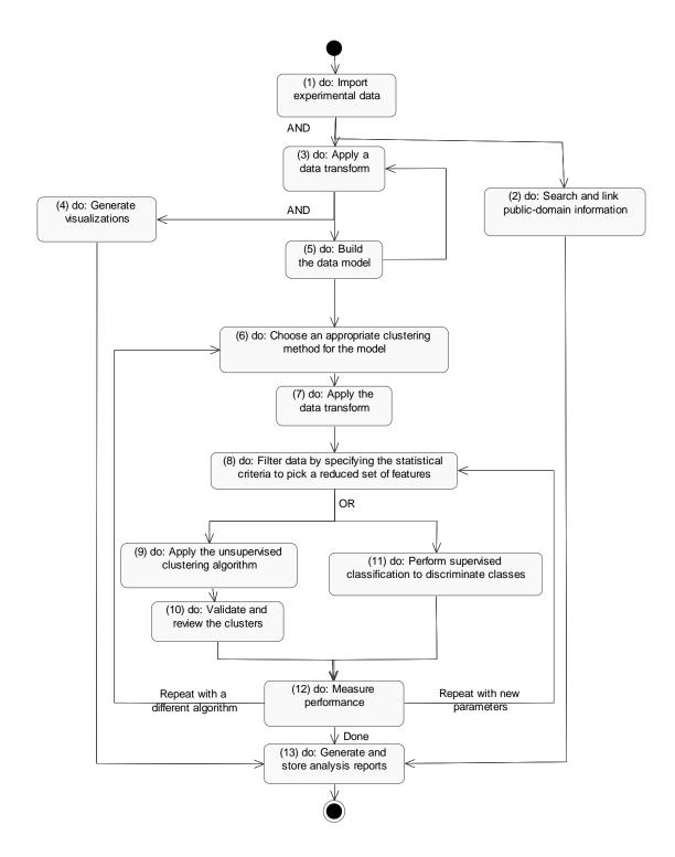
Fig. 4.12 State-chart Diagram for Behavior
