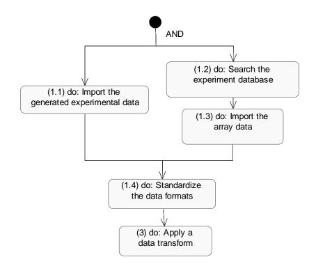
Fig. 4.14 Lower-level FFBD for Function 1: Import Experimental Data
