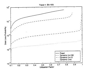
Figure 7: Performance of the dynamic link bandwidth allocation scheme.
