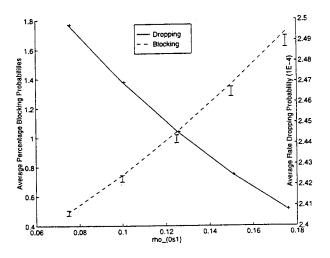
Figure 5: Tradeoff between call blocking and rate dropping probabilities.
