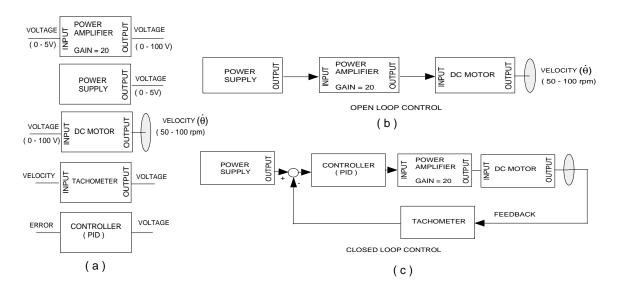
Figure 5: Figure 5: An example of a control system. (a) Components of the control system. (b) Open-loop control. (c) Closed-loop control.
