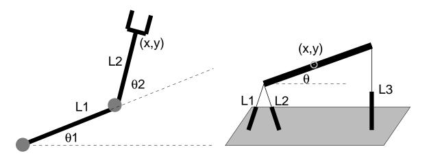
Figure 2: Manipulators used for kinematics problems: two-link serial planar manipulator (left) and parallel planar manipulator (right).
